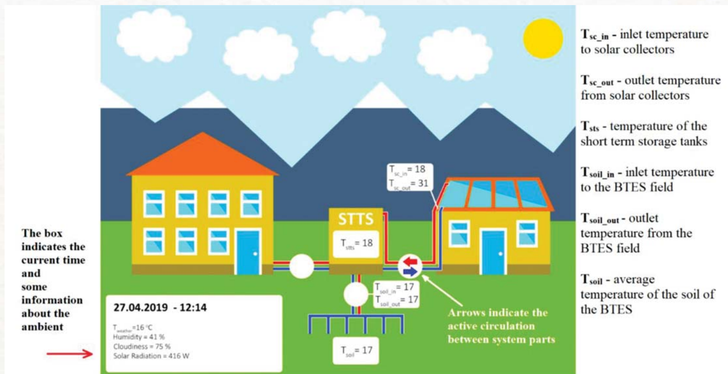
Temperature component and operating mode of SASTE technologies in the daytime in the Agrobiocenter
