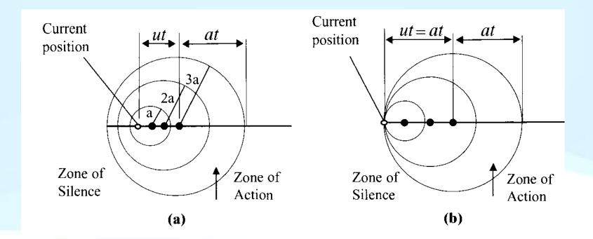
by the sound wave are tangent to the vertical line at the position of the observer. For supersonic speed, M > 1, the velocity of the body is faster than the speed of sound. The line tangent to the circles of the speed of sound, known as a Mach wave, forms the boundary between the zones of silence (outside) and action (inside). Only after the body has passed by does the observer become aware of it.
